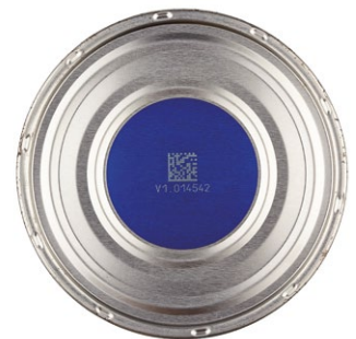
Color removal of DataMatrix code on metal
